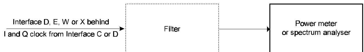
Figure E.4: Test set-up for RF/IF power measurement
