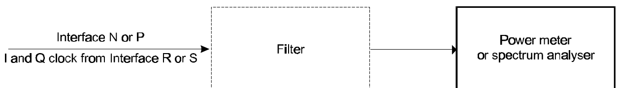
Figure B.8: Test set-up or out-of-service noise level measurement
