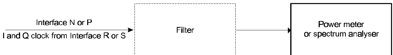
Figure B.7: Test set-up for RF/IF level measurement
