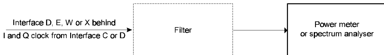
Figure E.5: Test set-up for out-of-service noise power measurement
